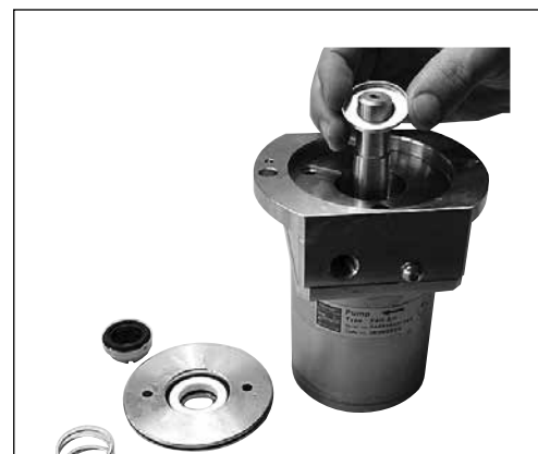
23. Mount the washer with the edge pointing upwards.
