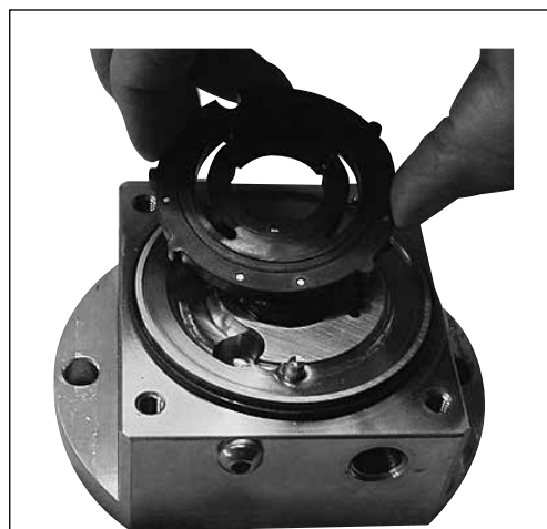
16. Remove the port plate from the flange.
