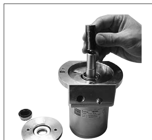
25. Fit the hollow bush onto the shaft.
